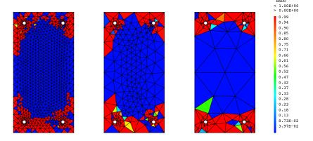
Figure 7: Damage fields obtained after optimization of the projection using the diffuse approximation.
