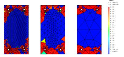
Figure 5: Damage fields obtained after optimization of the projection using the shape functions.
