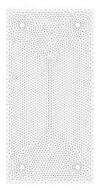
Figure 1: Fine mesh for the computation of the CS damage due to the rebars corrosion.
