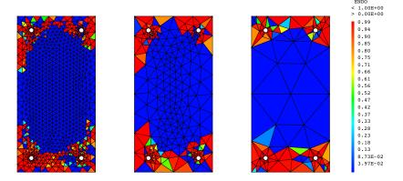
Figure 6: Damage fields obtained after projection by the method based upon the diffuse approximation, using 3 neighboring points.
