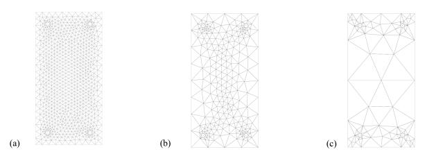
Figure 3: Coarser meshes used to test the projection techniques. (a) Mesh 1: 1686 elements. (b) Mesh 2: 452 elements. (c) Mesh 3: 156 elements.
